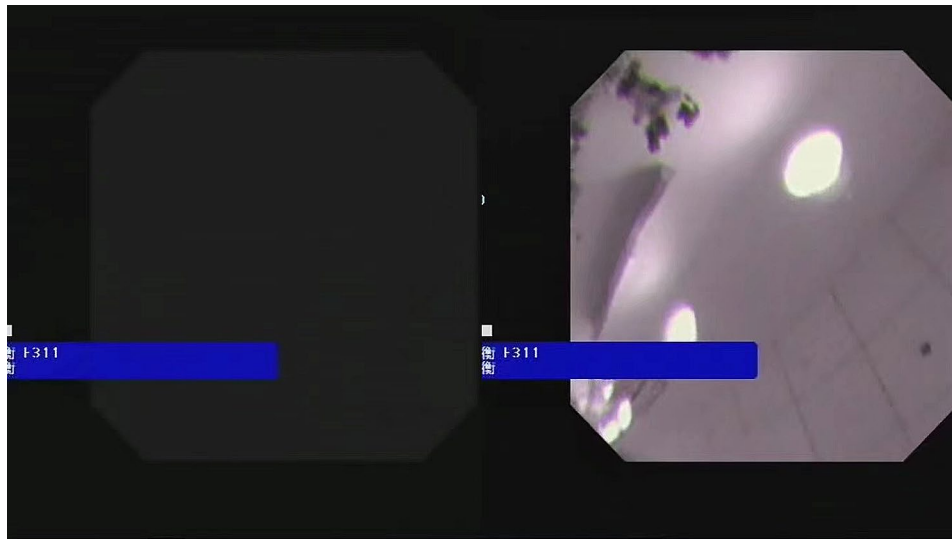
Fig. 1 No video image during angulation (left: no video image; right: image was being displayed)
