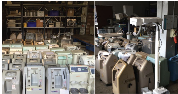
Fig. 1 Medical equipment graveyards in low-resource hospitals. Medical devices designed for use in high-resource settings often fail when used in harsh environmental conditions found in low-resource hospitals; because user instructions or spare parts are not accessible, broken devices remain in equipment graveyards like those pictured here in Malawi. Therefore, rigorous evaluation protocols are needed to identify medical devices that are effective, affordable, rugged, and easy to use in low-resource settings. (Photo credit: Brandon Martin, 2016)
