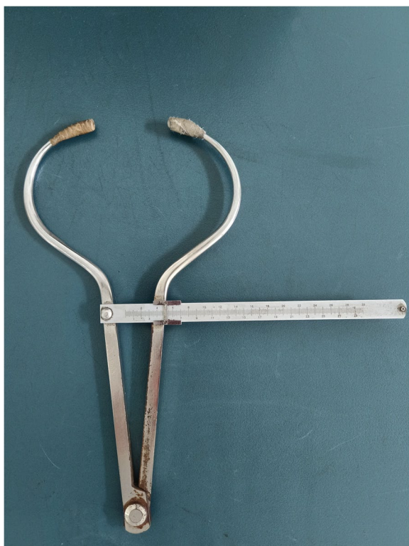
Fig. 1 The measurement tool was the KWJ124 bending foot gauge (size 260 × 260 + 36 mm), the measurement range was 0–300 mm, and the executive production standard was GB5704.3–85
